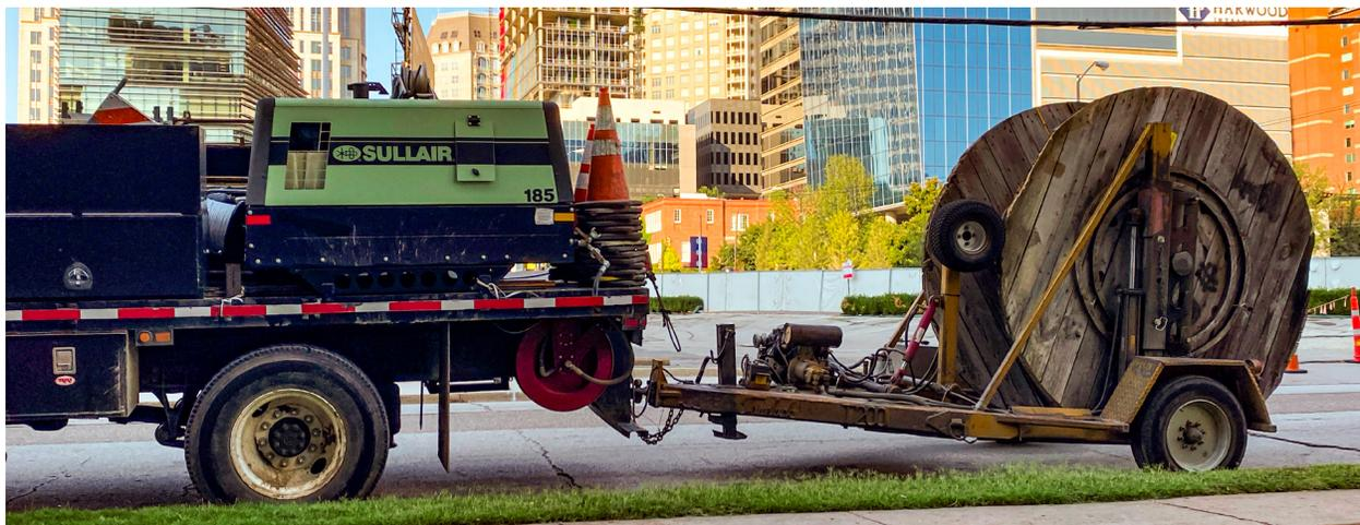
Compressed air is everywhere. Portable diesel air compressors bring compressed air wherever it is needed: plantside, roadside, refineryside and many other jobsites.
