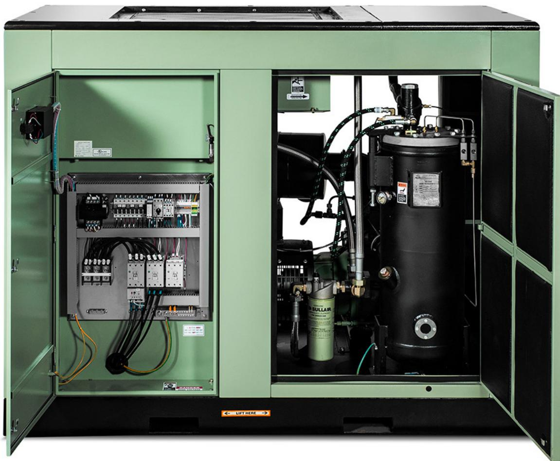
When selecting a rotary screw air compressor, there are two cooling configurations to choose from: air-cooled or water-cooled. Air compressors create a lot of heat during their normal operation. The heat comes mainly from the motor, air end and cooling circuit. Customers need to choose between an air-cooled or water-cooled compressor, and this decision is based upon the size, location and utilities available to the air compressor. Compressing air from 0 to 125 psig creates heat through
